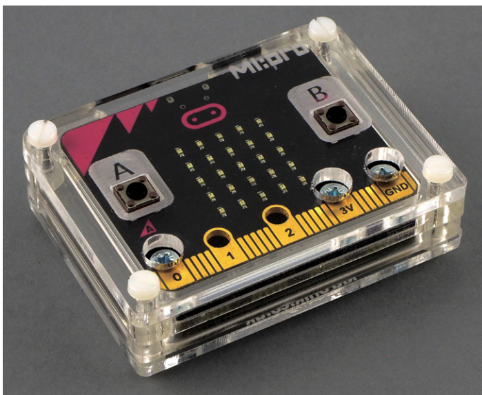
Figure 5-11: Kitronik Ml:pro case with Ml:power battery backpack
