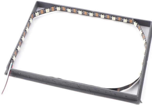
Figure 3-13: Attaching the LED strip to the plastic insert
