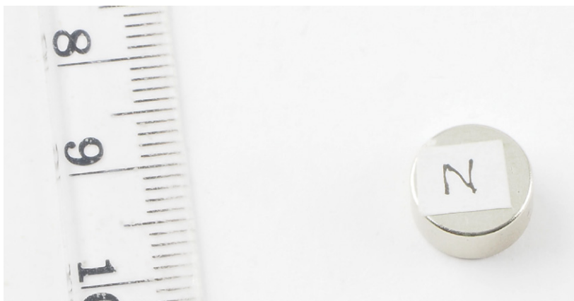
Figure 4-6: The neodymium magnet used for Experiment 4
